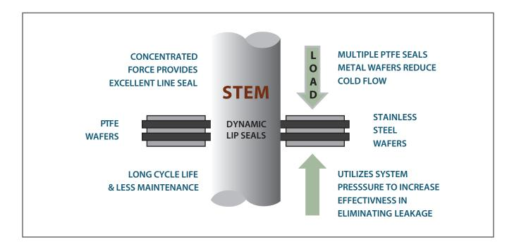
Dyna-Pak® provides superior sealing performance while reducing maintenance costs. Consisting of alternate wafers of PTFE and metal spacers, stem leakage is virtually eliminated while the problems associated with PTFE cold flow are minimized.
